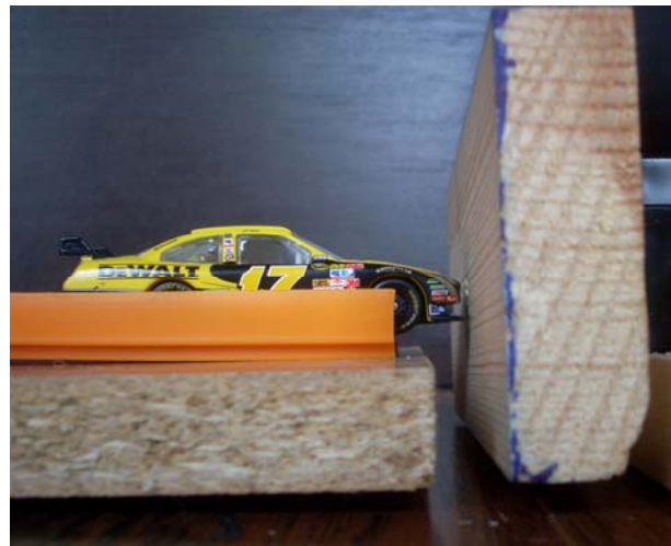
This is how the car should hit the wall. The part of the car that hits first should hit at approximately the center of the wall.
