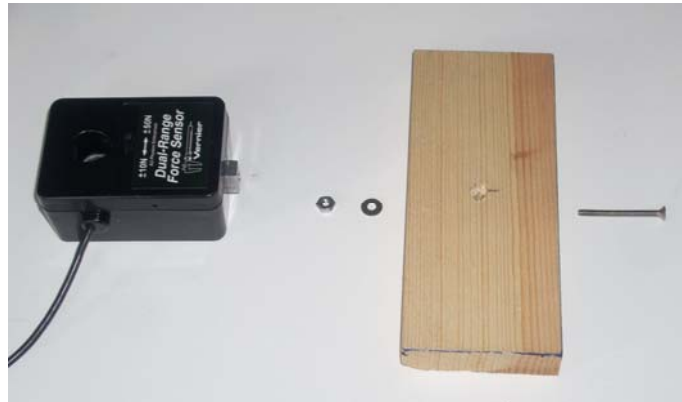
From left to right: The force sensor, a 6-32 nut, the washer for the 6-32 screw, a \frac{1}{2} " thick piece of plywood with a hole drilled through it, and the 1" long 6-32 screw.
