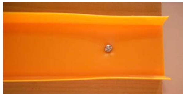
A screw holds the track to the plywood base at the end of the track.
